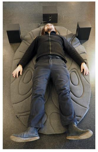
Figure 2 - Illustration of the speaker placement in relation to the user and mat (cabling has been omitted in this picture).
