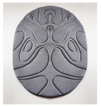
Figure 1 - Illustration of Sarka. The sewn patterns help align the body of the person lying down with the sensors underneath the mat. Cabling and speakers/headphones are not shown.
