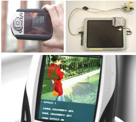
**Figure 1. Iterative prototyping: concept prototype (a); interaction prototype (b); camera phone prototype (c).**
