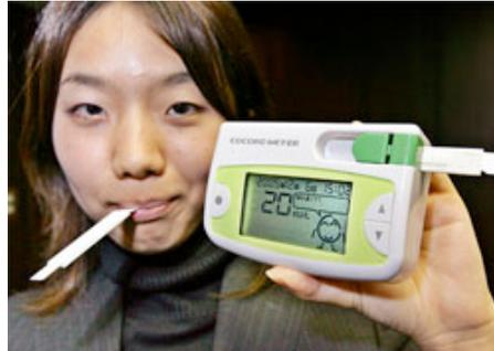
Fig. 2.4. The Cocoro saliva sampling system
