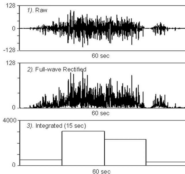
**Fig. 4.1.** Post processing of accelerometer. 1) Raw counts; 2) Rectified counts; 3) Epochs. Extracted from (Chen & Basset 2005)
