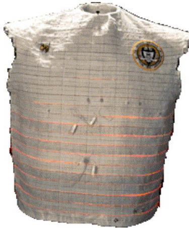
Fig. 2.8. Example of a smart textile called Georgia Tech Wearable Motherboard™
