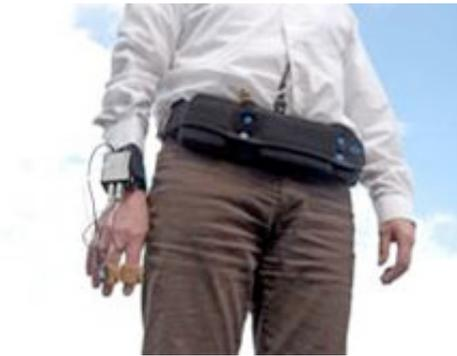
**Fig. 4.12.** Usage of Portapres. The sensors in the wrist and fingers communicate with the belt which has data storage capacity and a power source
