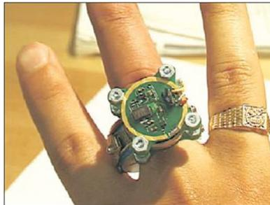
**Fig. 2.6.** Early prototype of a PPG ring
