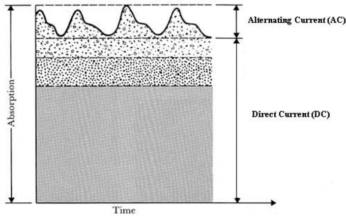
**Fig. 2.7.** Absorption of light by a PPG sensor. The AC part of the signal gives information about the heartbeat
