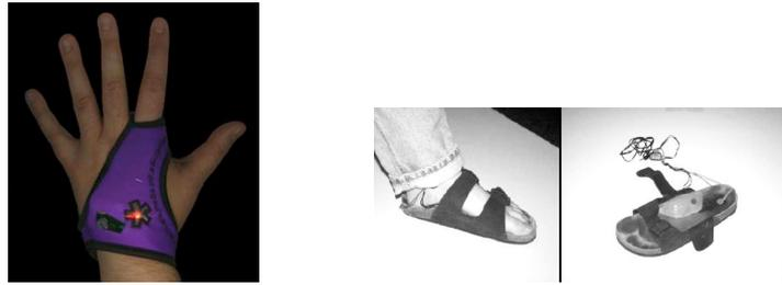
**Fig. 4.7.** Example of skin conductivity sensors in the hand and in the foot. Extracted from (Picard & Scheirer 2001) and (Picard & Healey 1997)
