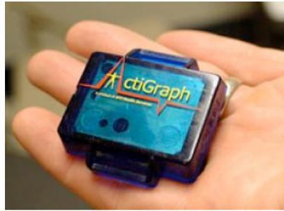
Fig. 4.2. Actigraph, an example of an accelerometer.
